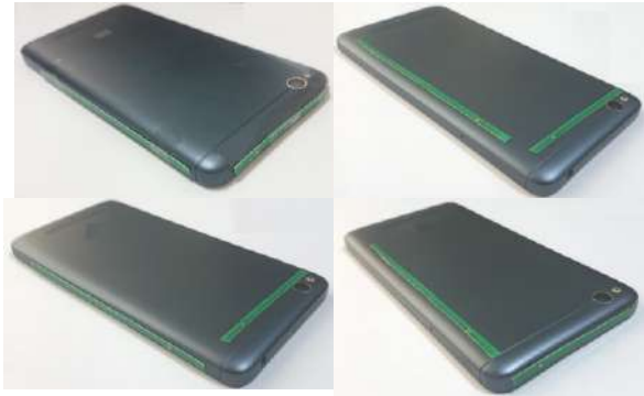
Fig. 8. Different configurations of MIMO antennas with a polarization diversity
