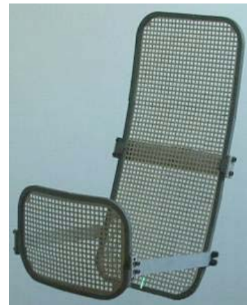
Fig.9 A prototype of the grid antenna with the new feed
