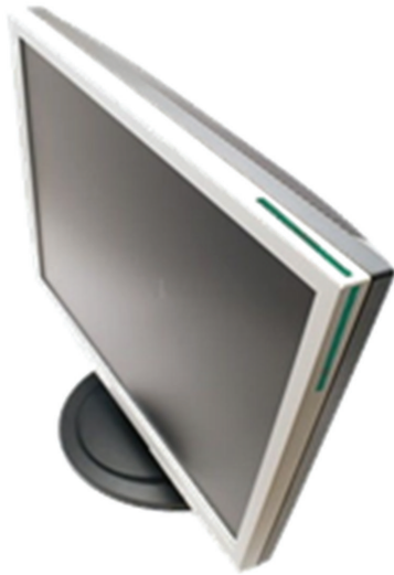
FIGURE 18: Two orthogonal antennas on a TV set with two different feed points for MIMO configurations.
