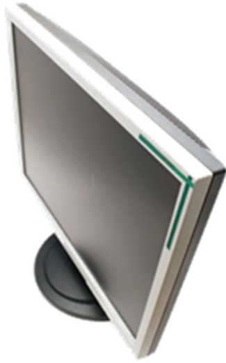
FIGURE 13: Two orthogonal antennas on a TV set with a common feed point.
