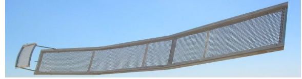
Fig.2 A prototype of gridded dual parabolic cylindrical reflectors
