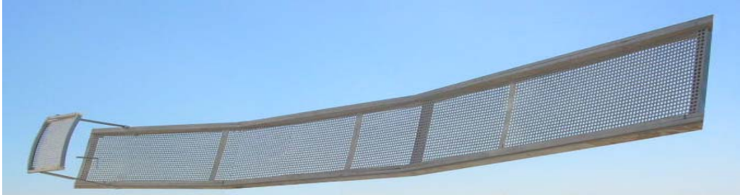
Fig.5 A prototype of grid dual parabolic cylindrical reflectors
