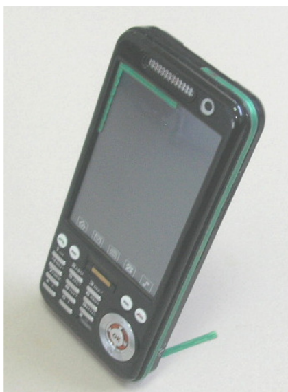
Fig.11 Bending the low-band antenna in three directions
