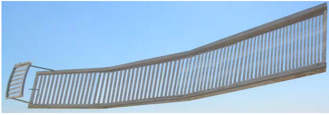
Fig.13 A prototype of the deployable / foldable antenna with the new feed
