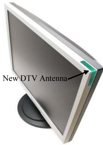
Fig.13 Optimum new antenna configuration on the display rim of a TV set
